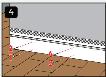
Secure trim in place with brad nails beginning furthest from **flange**.
