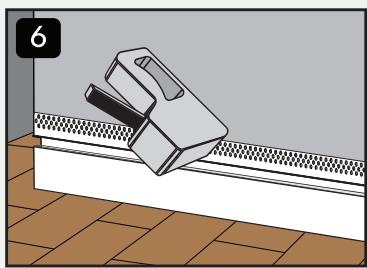
Once gluing is complete, add staples to the **flange** surface.
