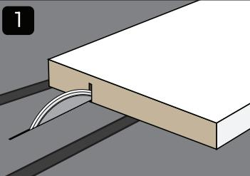
Cut a  $7/32$ " (6mm) slot in the rear of trim to the desired gap height.
