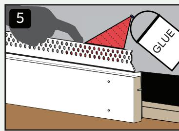
Peel **flange** forward and spray adhesive onto rear to ensure maximum bonding.
