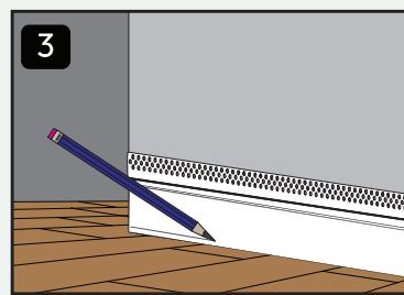
Dry fit **Flush Trim Mount** into drywall. Scribe trim to ensure flush finish.
