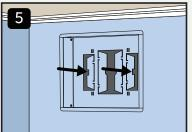
To adjust airflow, remove **plate** and bend dampers. For optimal air flow, push dampers past 90°.
