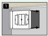
Dry-fit **body** into duct opening.
